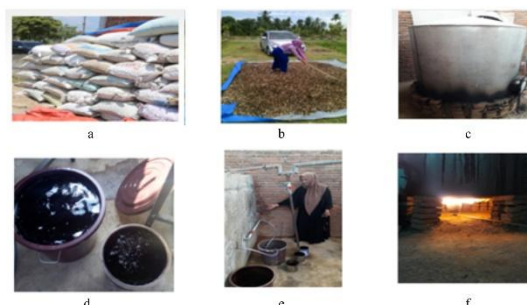
Figure 4. Liquid smoke production process using the pyrolysis method: (a) Candlenut shells collected as raw material; (b) The initial drying and preparation of the candlenut shells; (c) The batch pyrolysis reactor unit; (d) The collected grade 3 liquid smoke product; (e) Collection of the liquid smoke distillate from the
