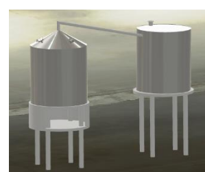
Figure 3. The designed and fabricated pyrolysis equipment used for liquid smoke purification study
