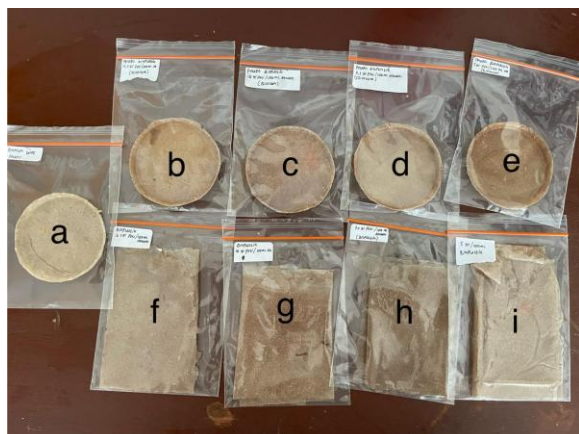
Figure 1. Visual appearance of biofoam and jackfruit seed starch bioplastic samples with different formulations (a) uncoated biofoam; (b) biofoam coated with 12.5 g JSS; (c) biofoam coated with 10 g JSS; (d) biofoam coated with 7.5 g JSS; (e) biofoam coated with 5 g JSS; (f) bioplastic sheet with 12.5 g JSS; (g) bioplastic sheet with 10 g JSS; (h) bioplastic sheet with 7.5 g JSS; and (i) bioplastic sheet with 5 g JSS.
