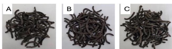
Figure 7. Physical appearance of RDF-5 pellets produced after biodrying under aeration rates of 0 L min -1 (A), 6 L min -1 (B), and 8 L min -1 (C).
