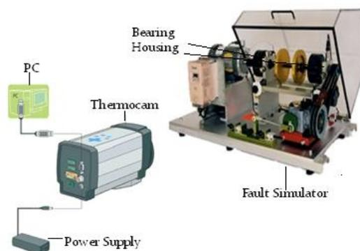
Gambar 2. *Machine Fault Simulator*
