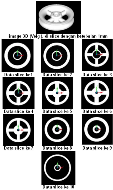
Figure 7. Sample Part and Its Sections
