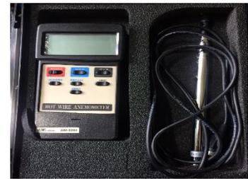
**Gambar 8.** Hot Wire Anemometer
