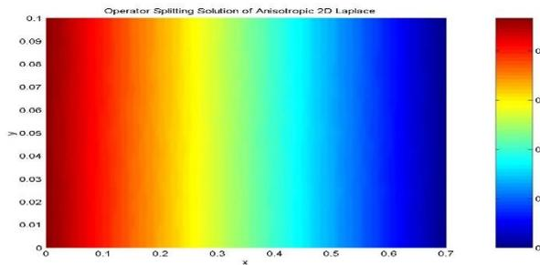
**Gambar 6.** OSM solution of anisotropic 2D Laplace's equation for  $\sigma_x = 3\sigma_y$ .
