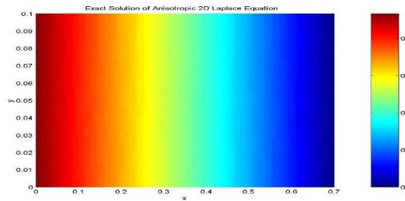
**Gambar 5.** Analytical solution of anisotropic 2D Laplace's equation for  $\sigma_x = 3\sigma_y$ .
