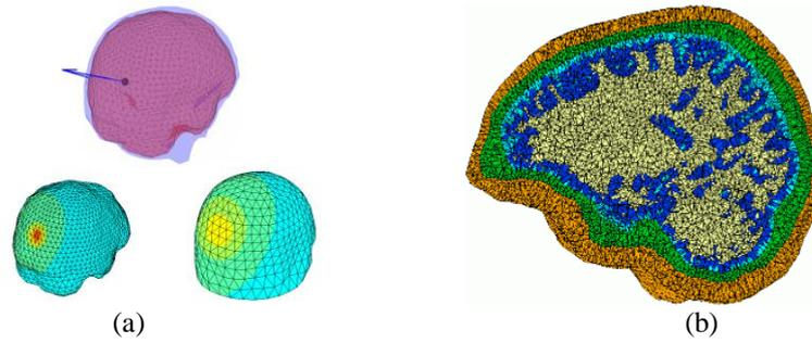
**Gambar 2.** (a) Human head model through triangle BE (b) Human head model through tetrahedral FE.
