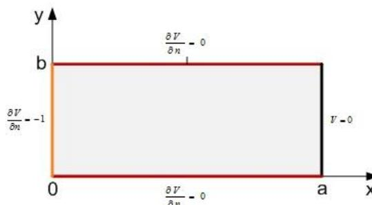
Gambar 3. Boundary conditions on the domain of 2D Laplace's equation.
