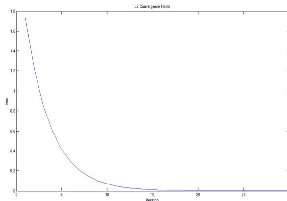
**Gambar 8.** Convergence rate of OSM in solving anisotropic 2D Laplace's equation for  $\lambda = 0.1$ ,  $n = 30$ .
