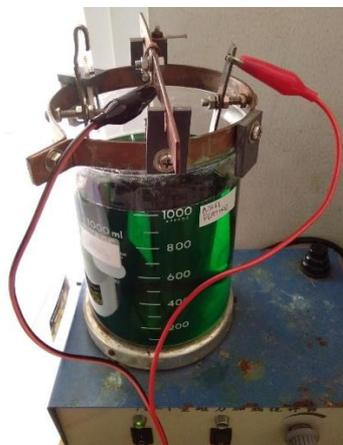
**Gambar 9** Proses elektroplating nikel
