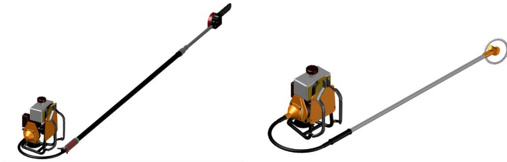
Gambar 1. Rancangan mesin potong model chainsaw blade dan circular saw blade
