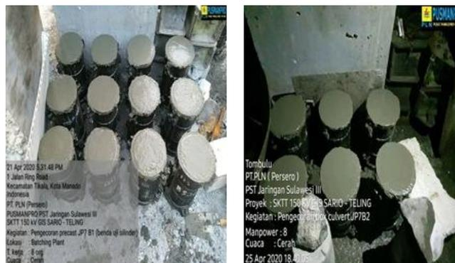
Gambar 7. Benda Uji Box Culvert Joint Pit (Sumber: PLN)
