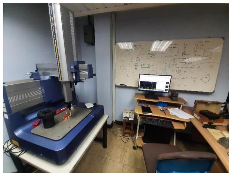
**Figure 3.** (a) Measurement position on the cube specimen for each surface, and (b) Setup using CMM machine
