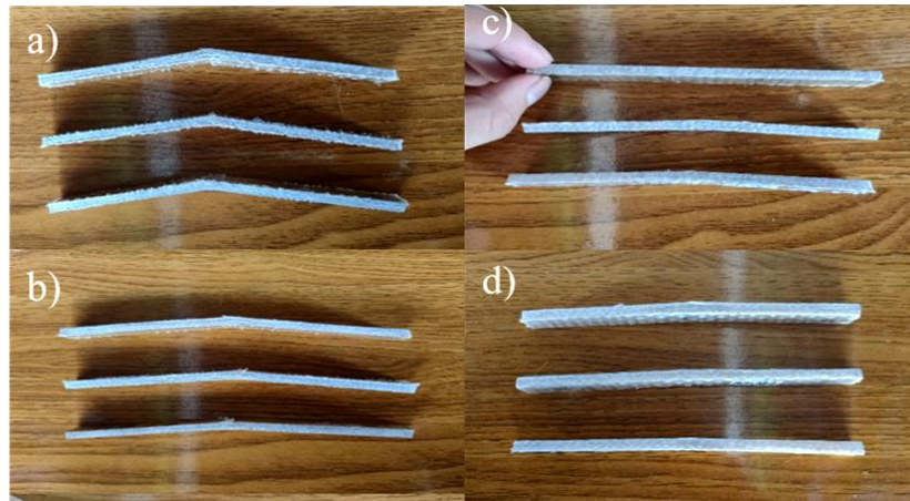
Figure 5. Hybrid composite after flexural test a) R–F–R–F–R Ramie 90° dan Fiber 45°, b) R–F–R–F–R Ramie 90° dan Fiber 60°, c) F–R–F–R–F Fiber 90° dan Ramie 45°, d) F–R–F–R–F Fiber 90° dan Ramie 60°.
