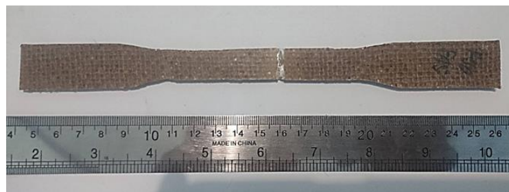
Figure 2. Post-test tensile specimen.
