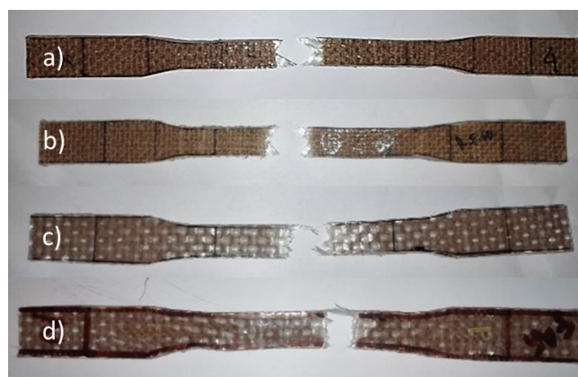
Figure 3. Fractured specimens showing pull out of the fiberglass layer. a) R-F-R-F-R, R90°/F45°, b) R-F-R-F-R, R90°/F60° c) F-R-F-R-F F90°/R60°, d) F-R-F-R-F F90° R45°.
