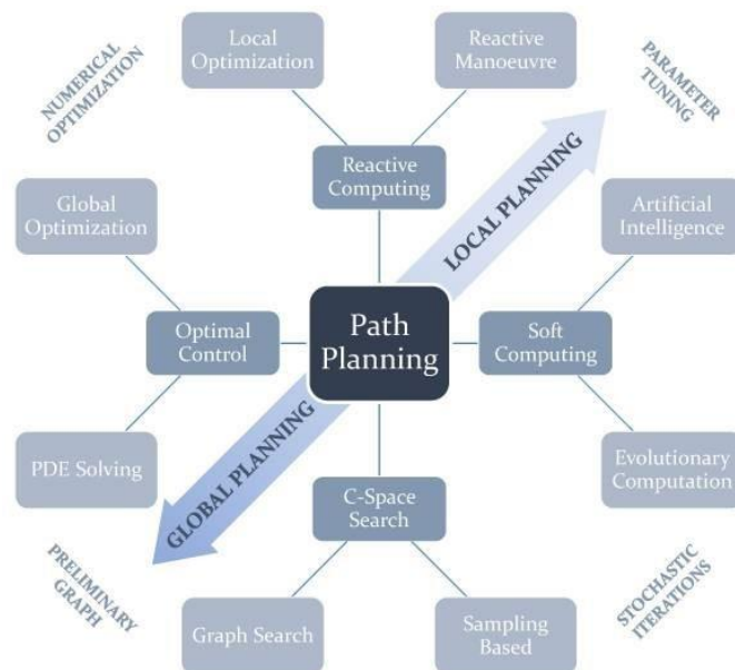
Figure 1. Proposed classification of existing path planning approaches [39]. Ant Colony approach is a sub-category of evolutionary computation (meta-heuristic) together with Genetic Algorithm, Memetic Algorithm, etc.
