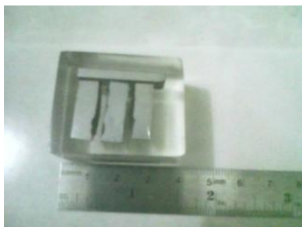
Gambar 3. Spesimen pengujian a). Axle Cotter b). Axle Bolt c). Axle Nut
