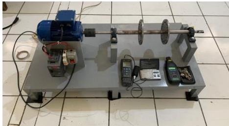
Gambar 2. Alat Uji *Two-Plane Dynamic Balancing*
