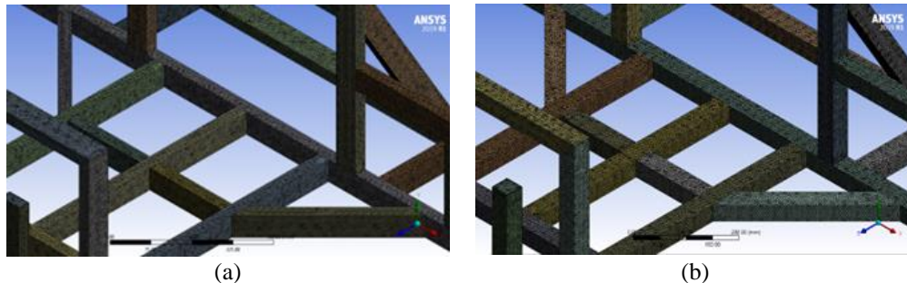
Gambar 2. Tetrahedron Element Mesh (a) Chassis Rectangular hollow, (b) Chassis Square Hollow
