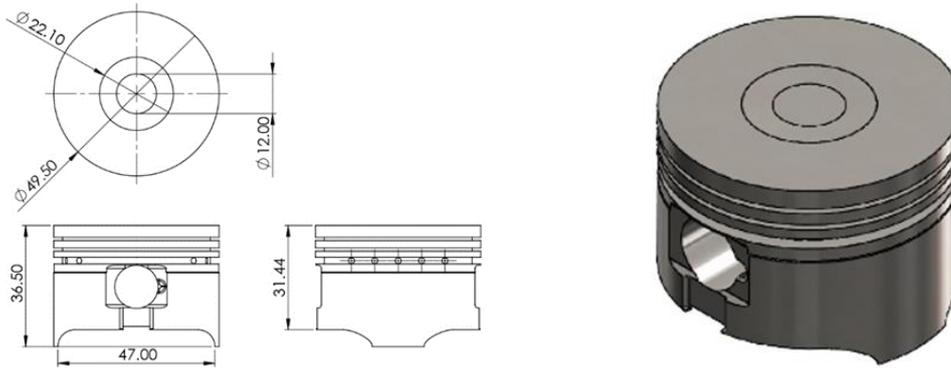
**Figure 1.** Honda Revo F1 2014 piston head dimensions
