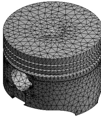
Figure 3. Mesh on piston head
