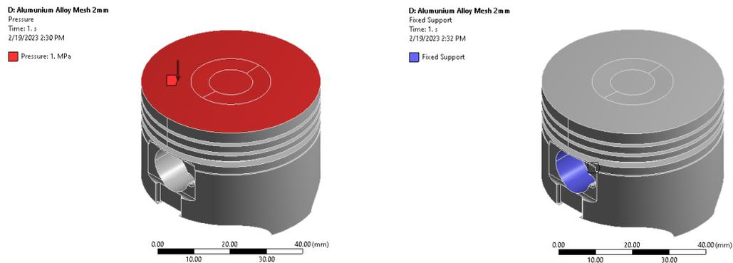
**Figure 2.** Provision of fixed support on the piston head
