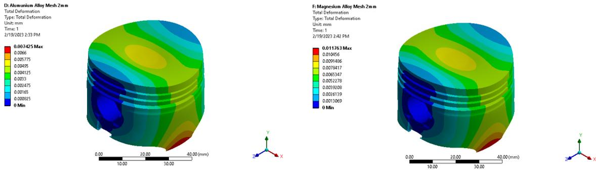
Figure 5. Total deformation in aluminium and magnesium alloys
