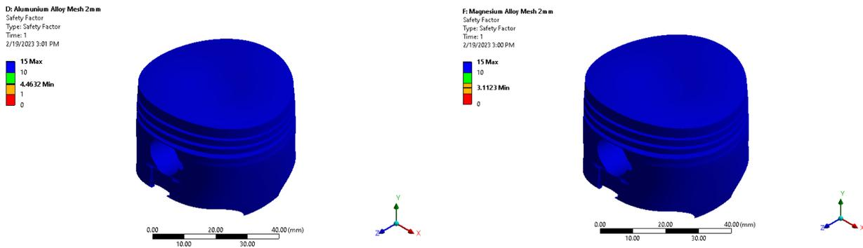
Figure 6. Safety factor of the piston head
