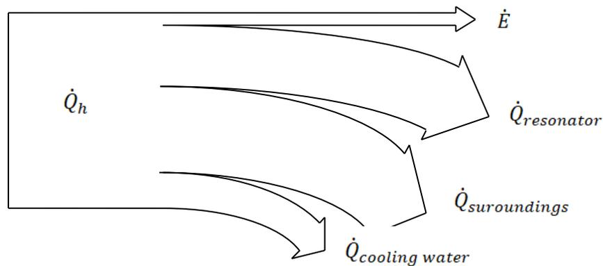
**Figure 12.** The Sankey Diagram of Conversion Thermal Energy to Acoustic and Losses Energy
