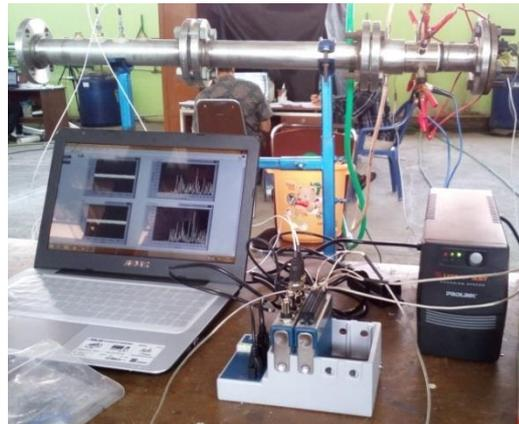
**Figure 6.** The Resonator length with 780 mm long
