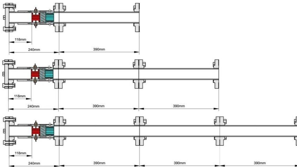
**Figure 4.** Three variations of resonator length of SWTE [10]
