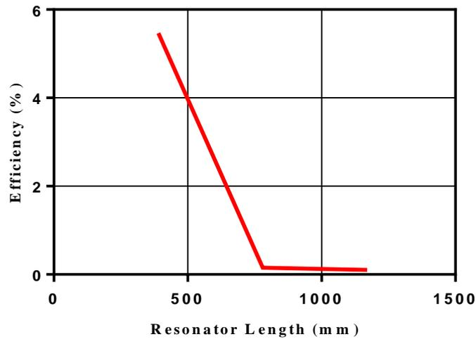
**Figure 11.** The Effect of Resonator Length toward Efficiency
