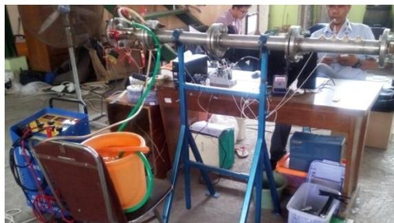
**Figure 7.** The resonator length with 1170 mm long
