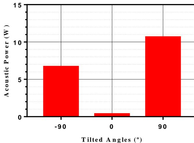
Figure 8. Effect of Tilted Angles toward Acoustic Power [9]
