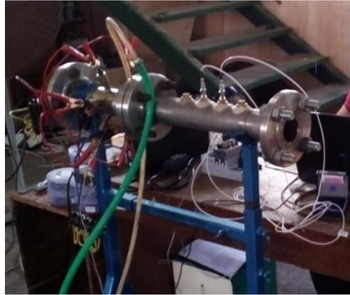
**Figure 5.** The resonator length with 390 mm long
