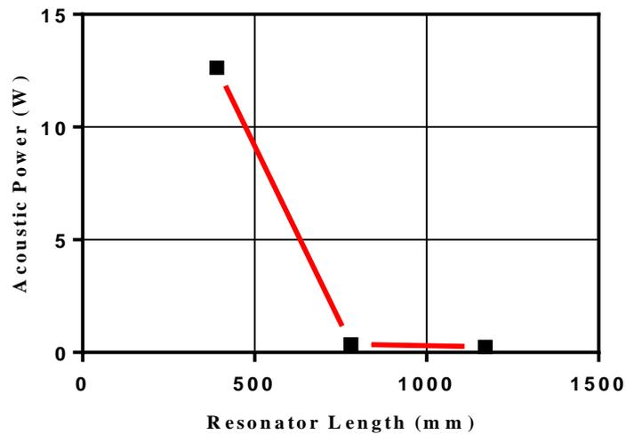
**Figure 9.** Effect of Resonator Length toward Acoustic Power
