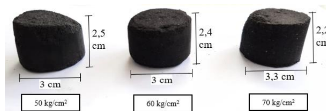
Figure 1. Charcoal briquettes with pressure variations
