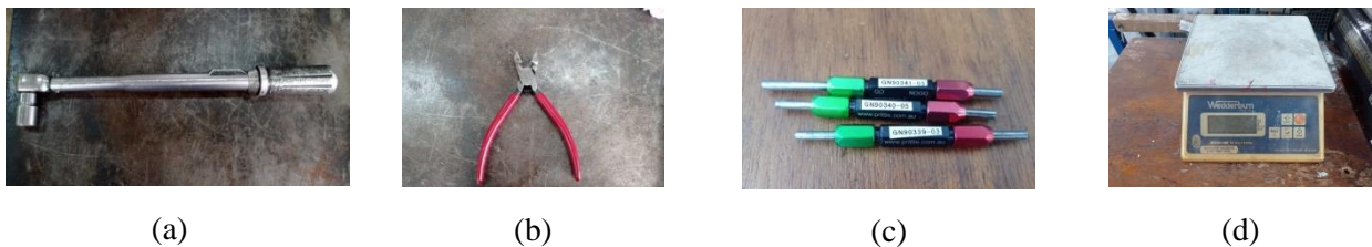
Figure 1: Tools for Injection Molding Process (a). Shock Keys (b) Cutting Tools (c) Plug Gauges, (d) Digital Scale
