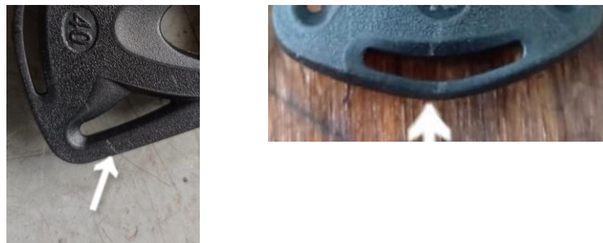
Figure 5. White Line Defect
