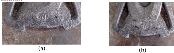
Figure 4. Short Mold Defect on (a) 2 nd Experiment (b) 3 rd Experiment
