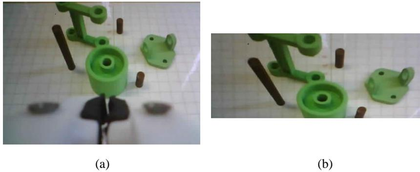
**Gambar 5.** Proses *Warping Frame* Kamera : (a) Sebelum *Warping*; (b) Sesudah *Warping*
