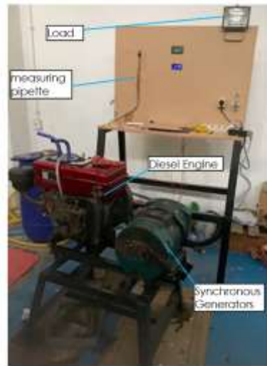
Figure 4. Engine Performance Testing Scheme
