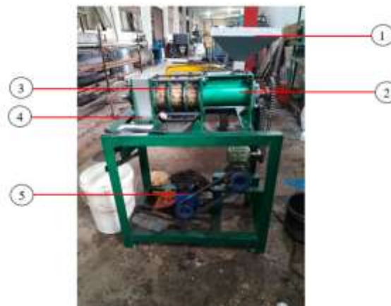
Figure 2. Screw press to extract crude oil from rubber seeds kernel
