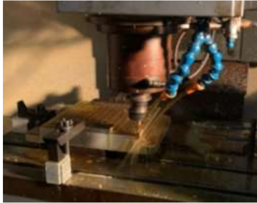
Figure 3. Side Milling Process
