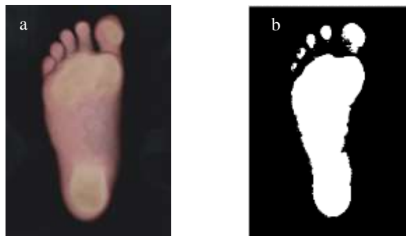
Figure 2.3 (a) Scanned Footprint at 300 DPI Resolution (b) Threshold Processing Result with an Index Level of 131
