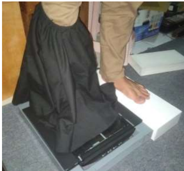
Figure 2.7 Foot Standing on the Scanner for Scanning Process with a Fabric Cover
