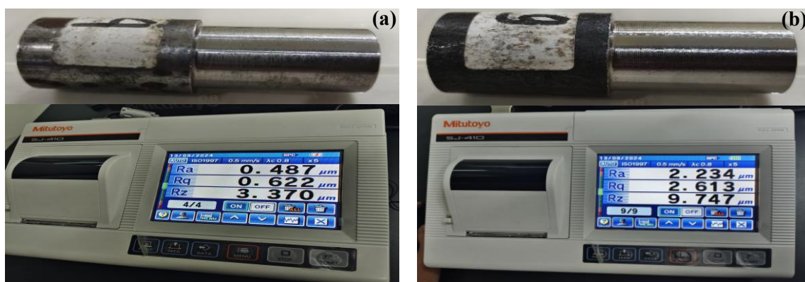
Figure 3. Cutting and Roughness test result: (a) Experiment 4, roughness 0.487 \mu\text{m} and (b) Experiment 9, roughness 2.234 \mu\text{m}
