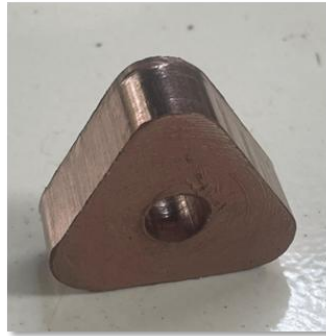
Gambar 5. Green compact brake pad
