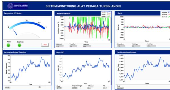
Gambar 6. Tampilan GUI Sistem Monitoring Alat Peraga Turbin Angin
