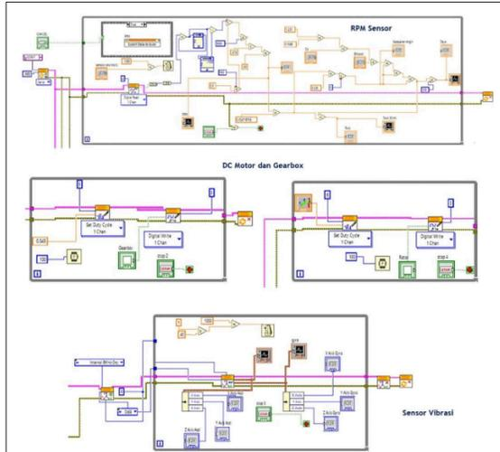
Gambar 7. Tampilan Virtual Instrumen (VI) Sistem Monitoring Alat Peraga Turbin Angin
