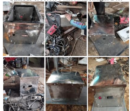
Figure 7. Aerator Frame Cover Manufacturing Process Gambar 7. Proses Pembuatan Penutup Rangka Aerator
