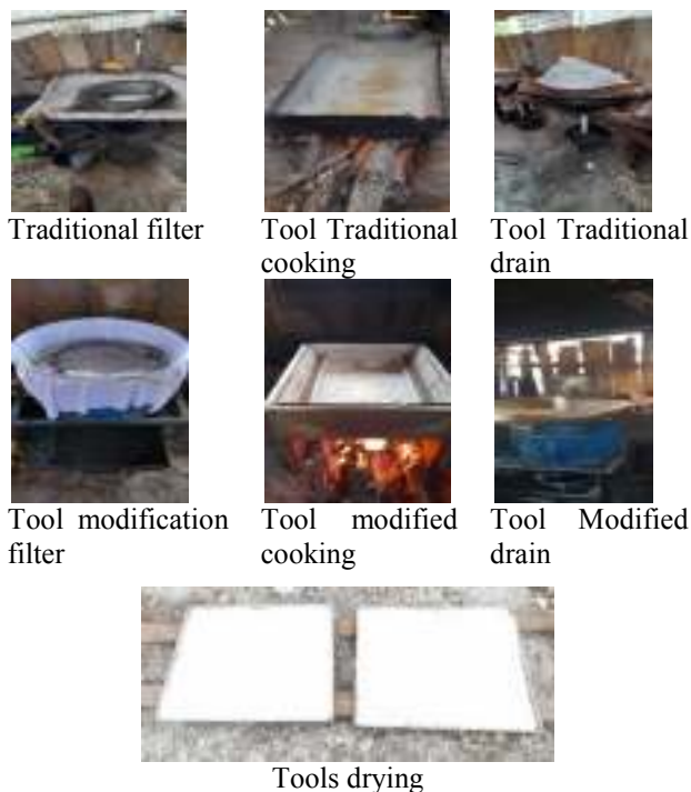
Figure 1. Equipment Traditional Salt Production and Equipment Modified Salt Production in the Tiberias Group, West Oesapa Village, Kelapa Lima District, Kupang City, East Nusa Tenggara Province.
