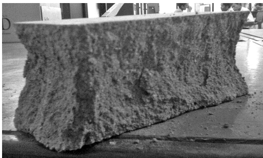
Figure 4. Cracking Pattern of Tested Paving Blocks
