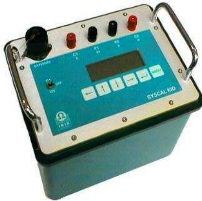
Gambar 4. Resistivity Meter, Syscal Kid Resistivity Meter serial RS232 ( Anonim, 2007b).
