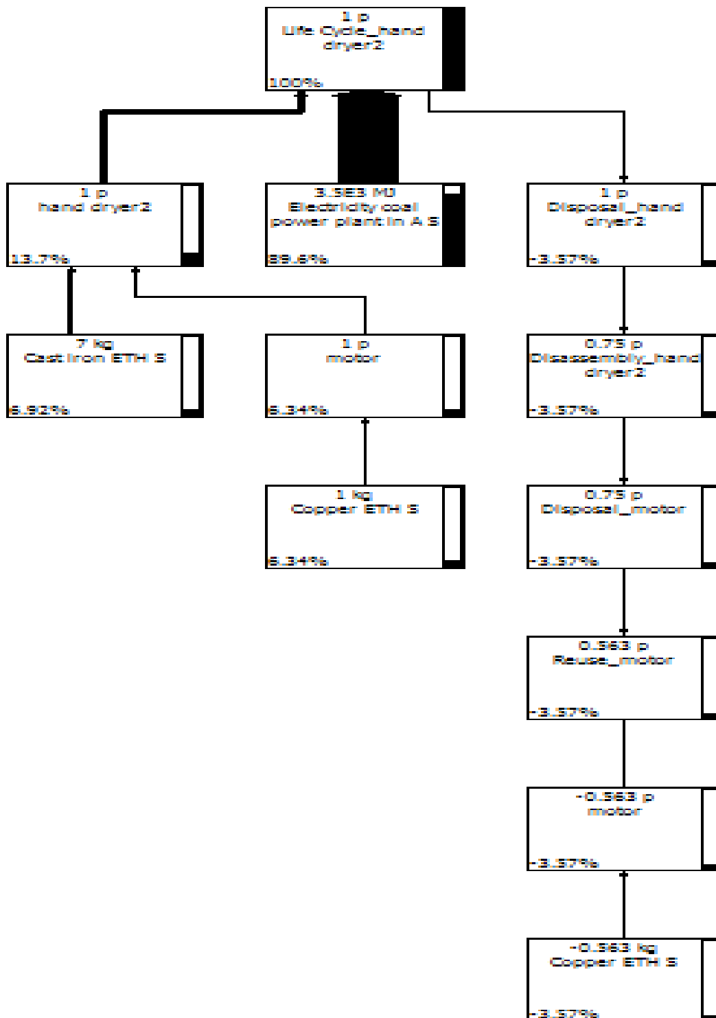
Figure 4 Flow diagram of electric hand dryer life cycle
