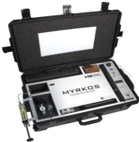
**Gambar 1.** Myrkos Portable DGA Micro GC (DGA Analyzer)
