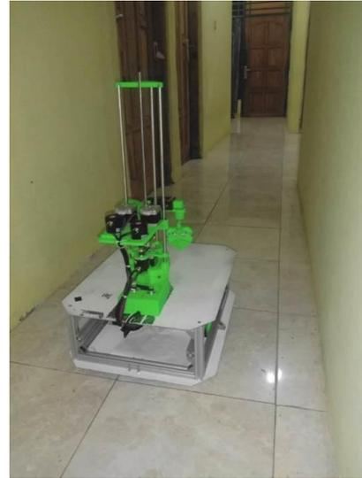
**Figure 5.** The mobile robotic arm navigates through the hallway to the room during the experimental environment.
