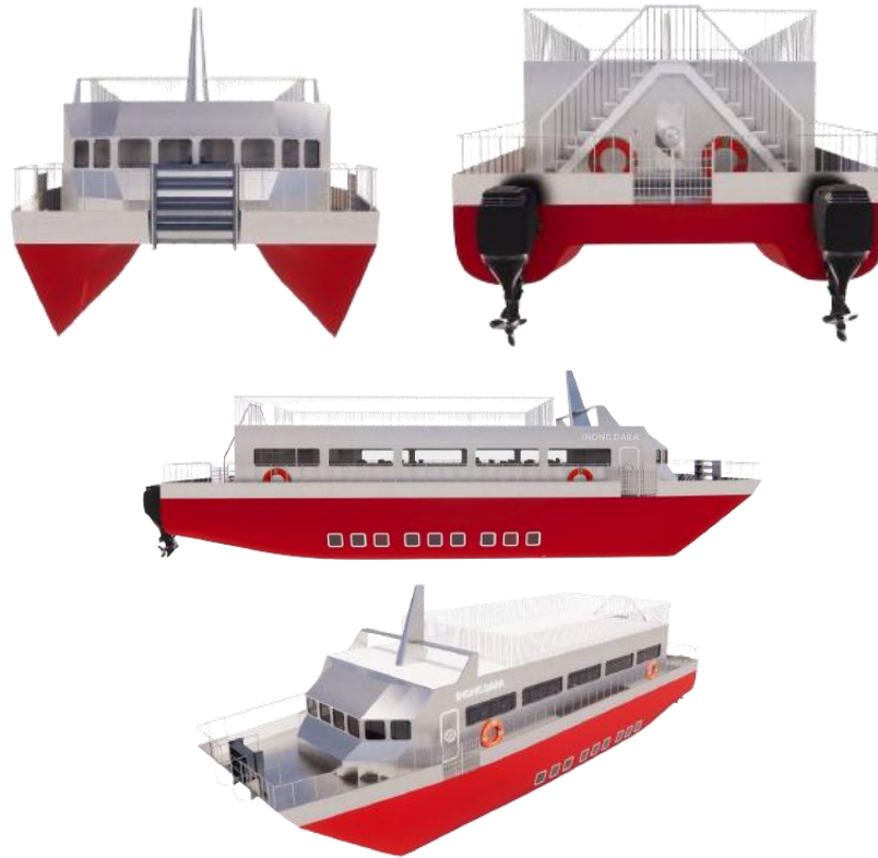
Figure 5. Designated 3D Glass Bottom Catamaran general arrangement plan
