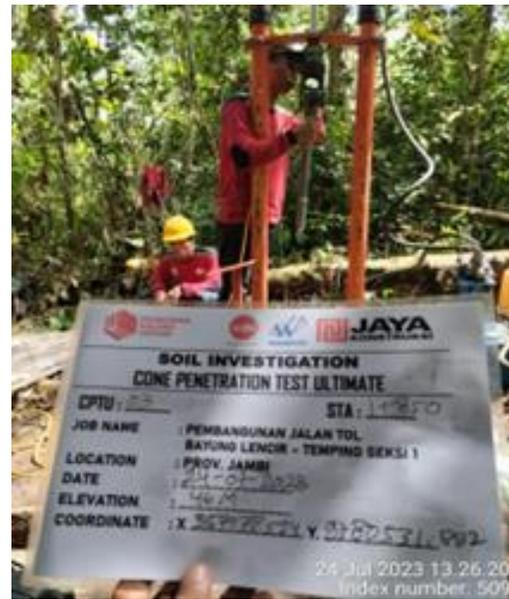
Gambar 7. Pengujian Cone Penetration Test Ultimate (CPTU)
