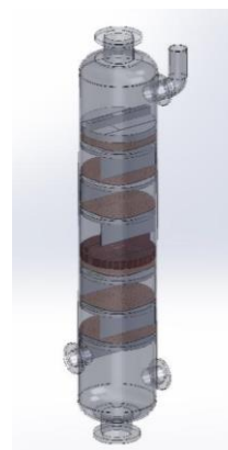
Figure 4. Configuration of A PVDF Membrane Distillation Tower Resulting from The Restructuring of A Conventional Distillation Tower
