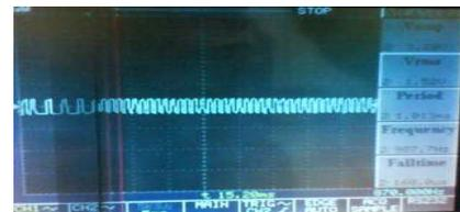
**Gambar 13 Deretan pulsa perintah Detonator B**
