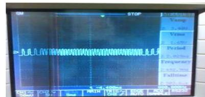
**Gambar 12 Deretan pulsa perintah Detonator A**
