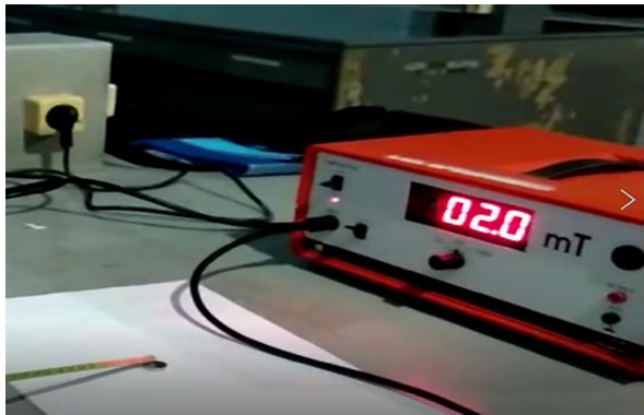
Gambar 10. Pengukuran densitas fluks magnet Neodymium Iron Boron (NdFeB)
