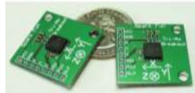
Gambar 2 Break out accelerometer MMA7260Q.
