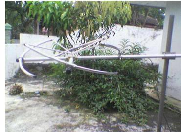
Gambar 10. Konstruksi real antena  $5/8\lambda$
