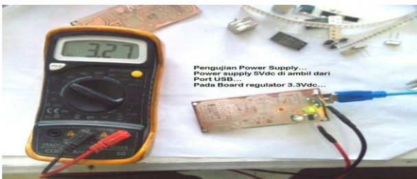
Gambar 5. Pengujian power supply
