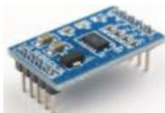
Gambar 5. Modul Sensor Accelerometer MMA7361
