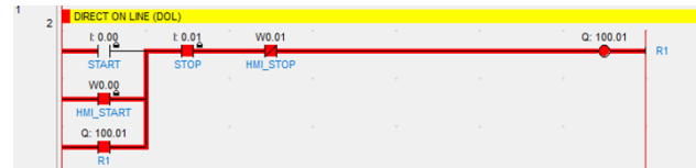
Gambar 7. Ladder Diagram Kontrol DOL melalui HMI
