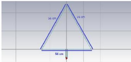
Gambar 1. Desain antenna *delta loop double band*
