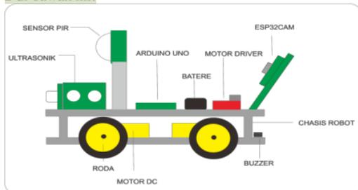
**Gambar 2. Rancangan Purwarupa Robot Mobile Beroda**
