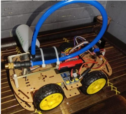
Gambar 4. Fabrikasi Purwarupa Robot Mobile Beroda
