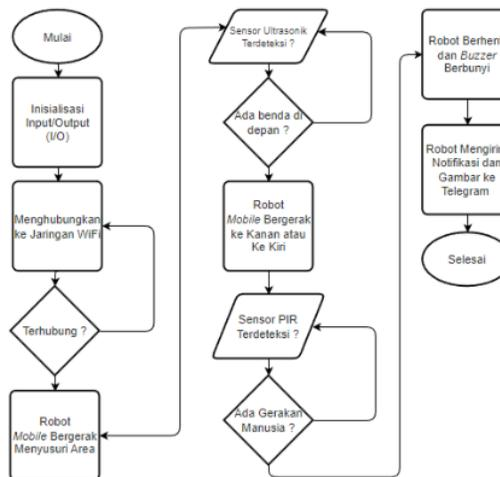
Gambar 1. Prinsip Kerja Robot *Mobile* Beroda
