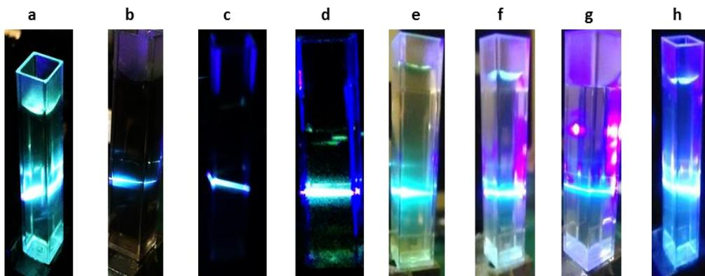
Figure 3. The physical appearance of CQDs emission from (a) DRL-CQDs-Hydrothermal, (b) FRL-CQDs-Hydrothermal, (c) DRL-CQDs-Microwave, (d) FRL-CQDs- Microwave, (e) DPL-CQDs-Hydrothermal, (f) FPL-CQDs-Hydrothermal, (g) DPL-CQDs-Microwave, (h) FPL-CQDs- Microwave
