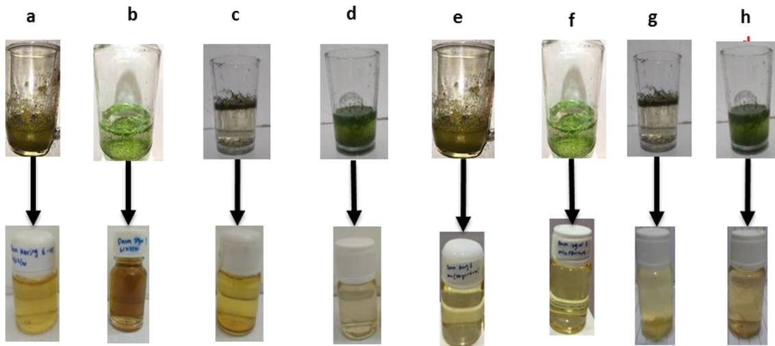
Figure 1. The physical appearance of CQDs from (a) DRL-CQDs-Hydrothermal, (b) FRL-CQDs-Hydrothermal, (c) DPL-CQDs-Hydrothermal, (d) FPL-CQDs-Hydrothermal, (e) DRL-CQDs-Microwave, (f) FRL-CQDs-Microwave, (g) DPL-CQDs-Microwave, and (h) FPL-CQDs-Microwave
