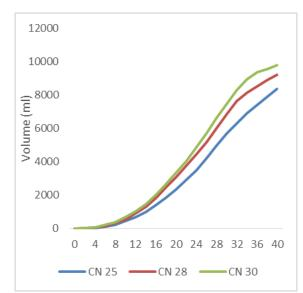
Figure 4. Accumulation of daily biogas production with C/N values of feed 25, 28, and 30 of the volume of biogas produced
