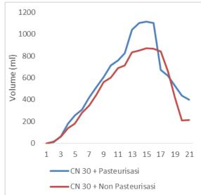
Figure 5. Daily biogas production with a C/N value of 30 feeds with pasteurization and without pasteurization on the volume of biogas produced
