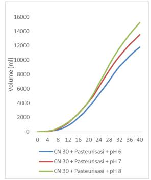
Figure 8. Accumulation of daily biogas production with pasteurized 30 C/N feeds with pH 6, 7, and 8 on the volume of biogas produced
