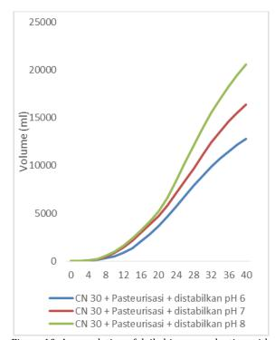
Figure 10. Accumulation of daily biogas production with pasteurized 30 C/N feed with a stable pH of 6, 7, and 8 on the volume of biogas produced
