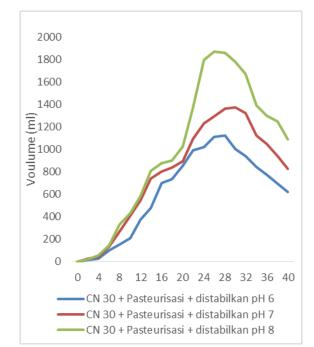
Figure 9. Daily biogas production with pasteurized 30 C/N feed with a stable pH of 6, 7, and 8 on the volume of biogas produced
