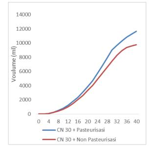
Figure 6. Accumulation of daily biogas production with C/N 30 feed through pasteurization and without pasteurization of the volume of biogas produced
