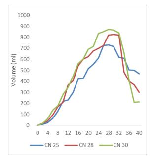
Figure 3. Daily biogas production with C/N values of 25, 28 and 30 feeds on the volume of biogas produced
