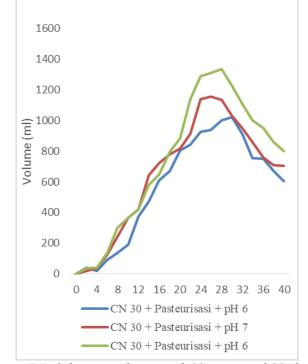
Figure 7. Daily biogas production with 30 pasteurized C/N feeds with pH 6, 7, and 8 on the volume of biogas produced
