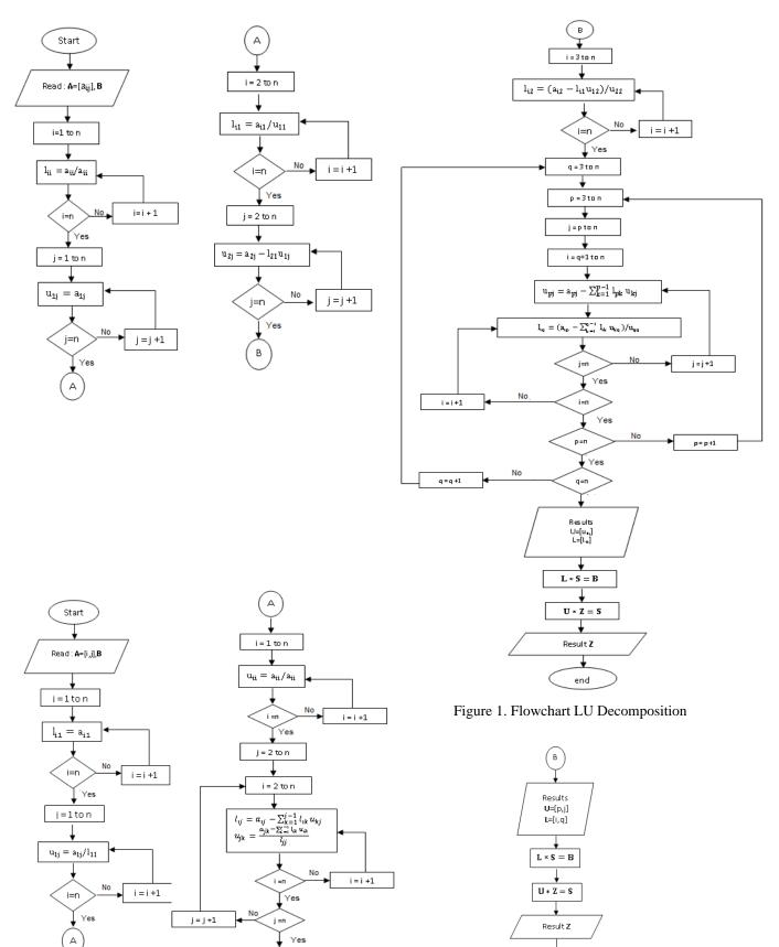
Figure 2. Flowchart Crout decomposition
