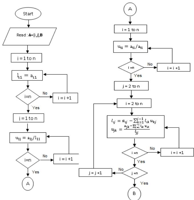
Figure 2. Flowchart Crout decomposition
